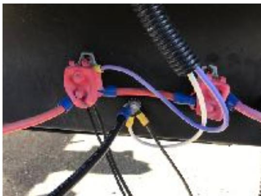
In this photo, the red wire is hooked to the breaker (fuse) which tells us that it is the positive. The black wire is attached to the frame of camper which means it is negative.
